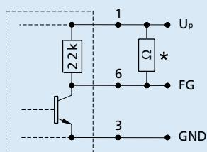
\* An additional external pull-up resistor can be added to improve the rise time.
